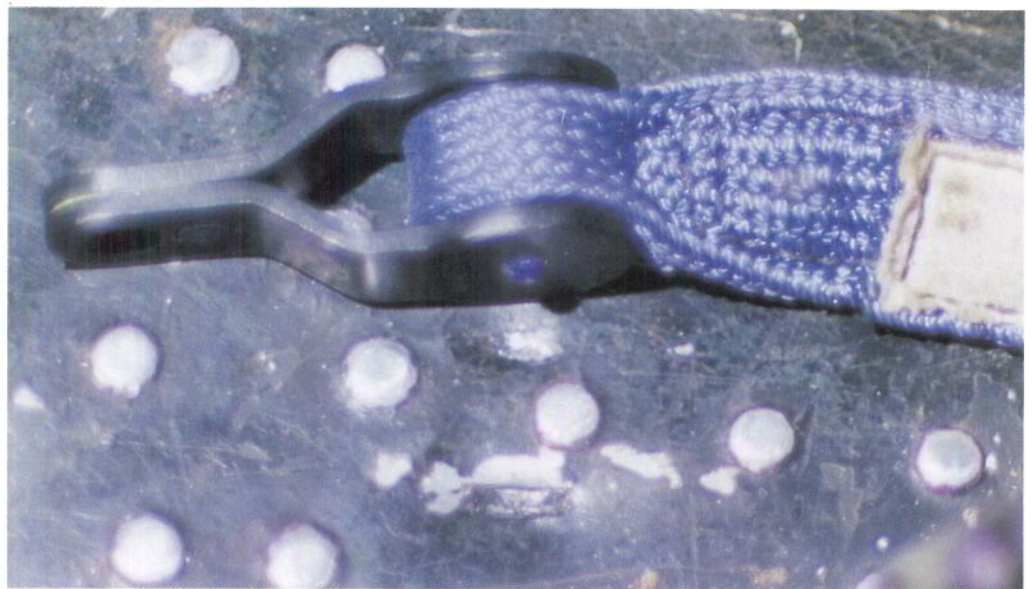
Plate 8 Dents on cockpit floor with leg restraint floor attachment fitting held beside it.
