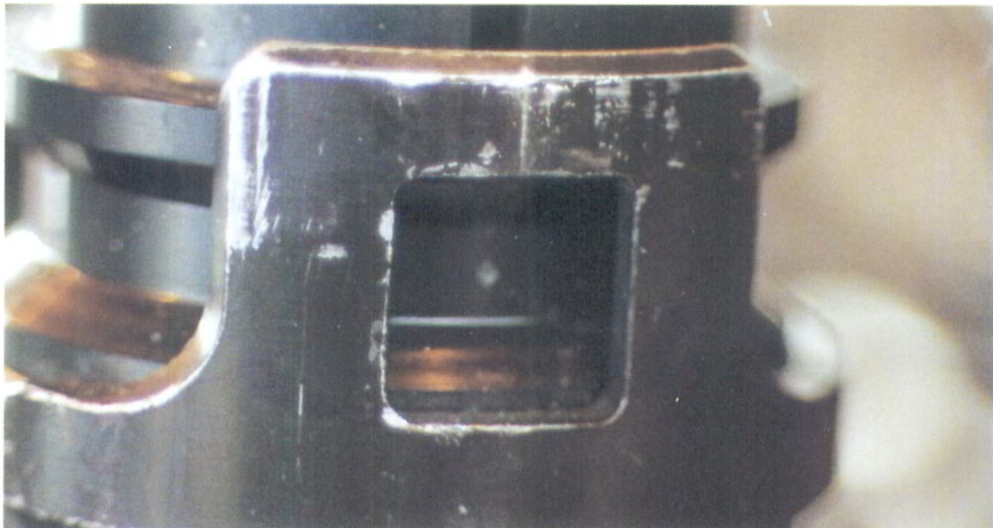
Plate 6 Latch window of left seat ejection gun
