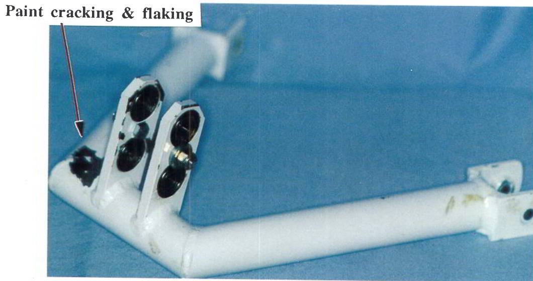
Figure 2 - Fork from flying control system of VPM M16, G-BVRD
