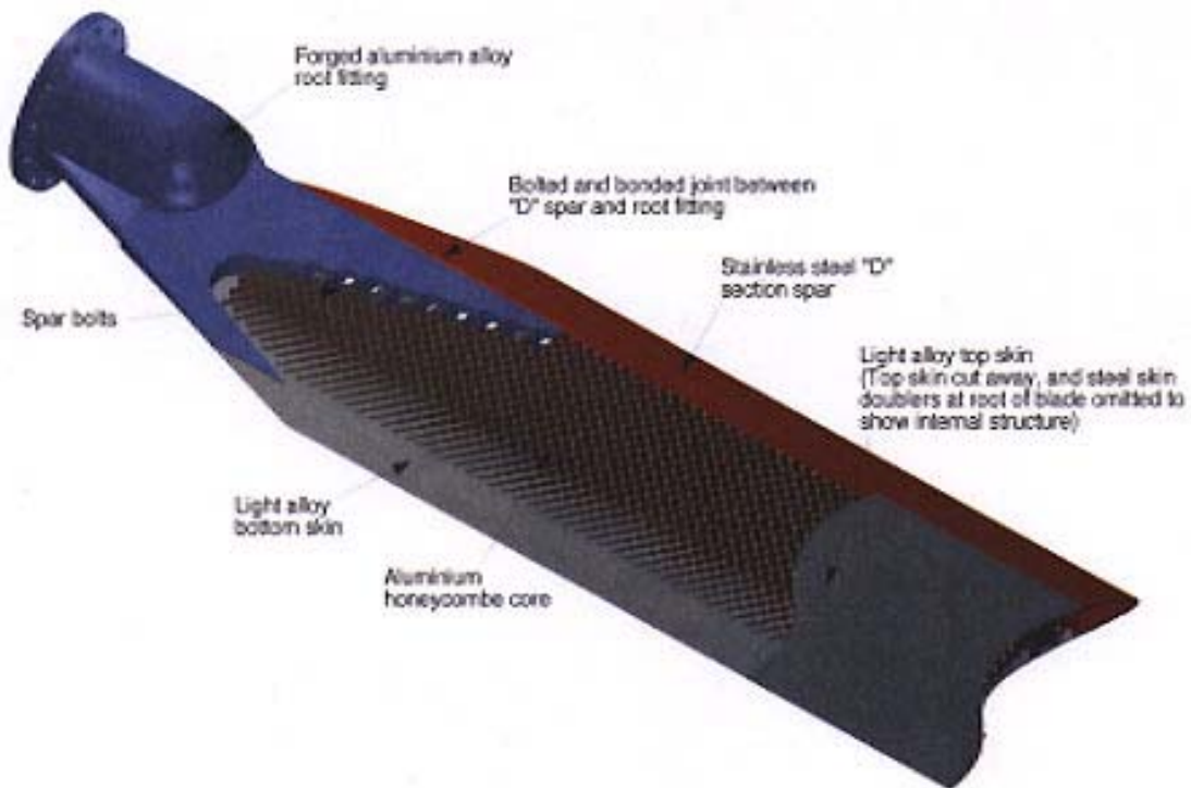
Figure 2a R22 Main rotor blade construction details
