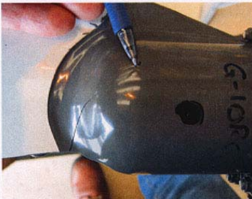
Figure 5 Topsurface crack (length approximately 7 cm)
