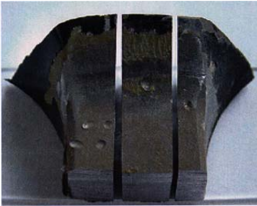
Figure 13 Surface condition of intact blade from G-IORG (Note: 'dingles' bruise marks are post-incident damage, from initial attempts to remove filler/adhesive)
