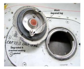
**Figure 1** Fuel filler cap
