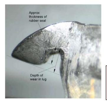
Figure 3 Illustration of wear in bayonet lug (viewed from the side)
