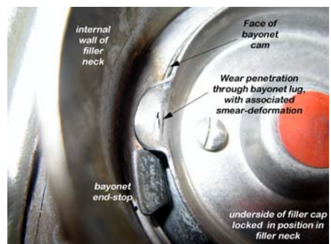
Figure 2 Underside of filler cap showing worn bayonet cams
