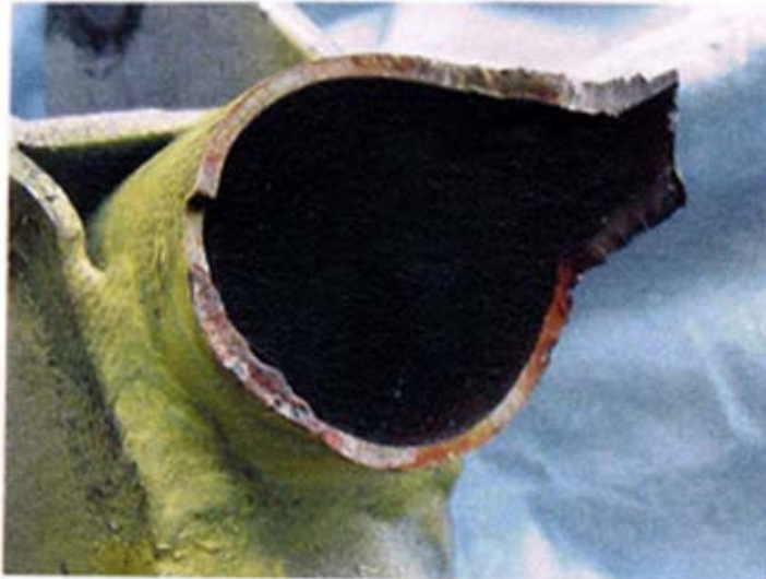
Detail of fatigue crack/overload fracture surface
