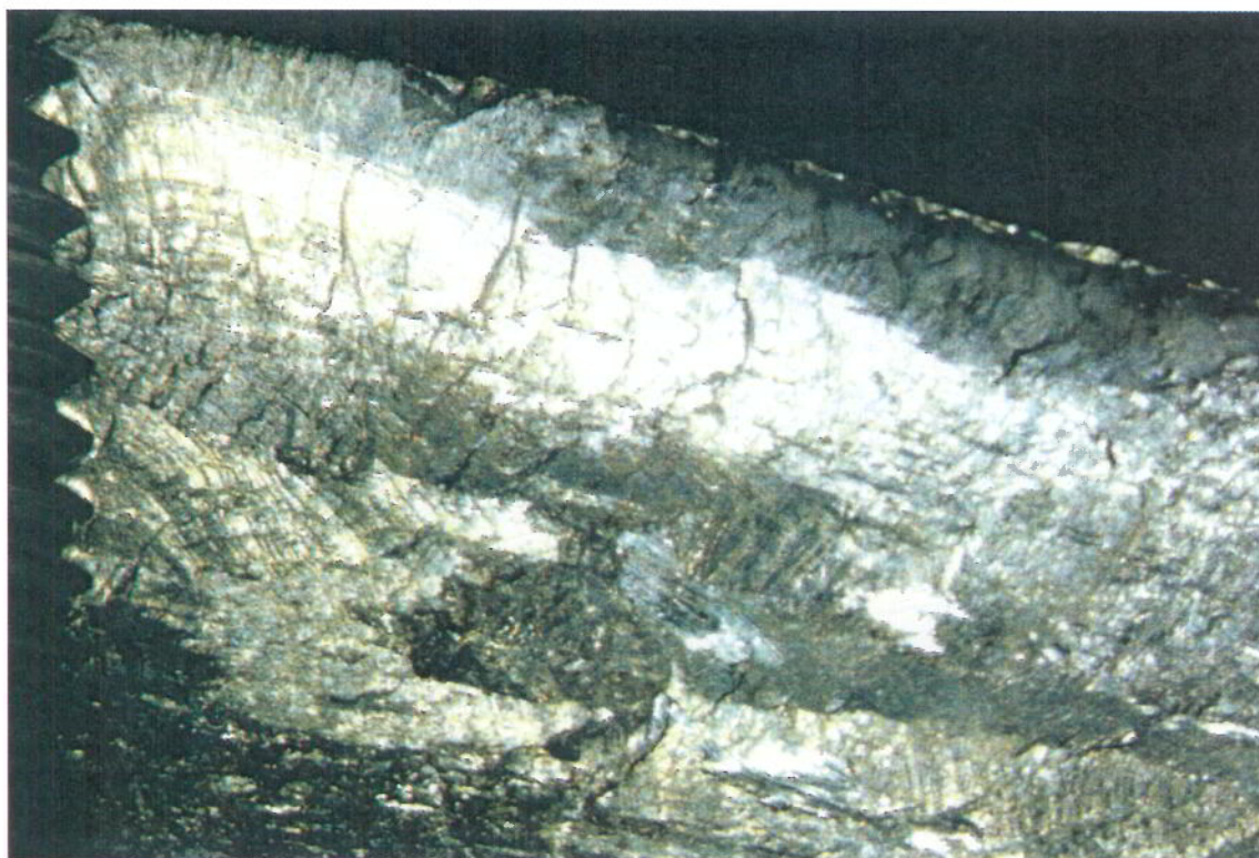
Figure 20 Typical view of the fatigue progression in the fracture face on the opposite side of the hole. The progression rates are very similar to those shown on figures 14 to 19
