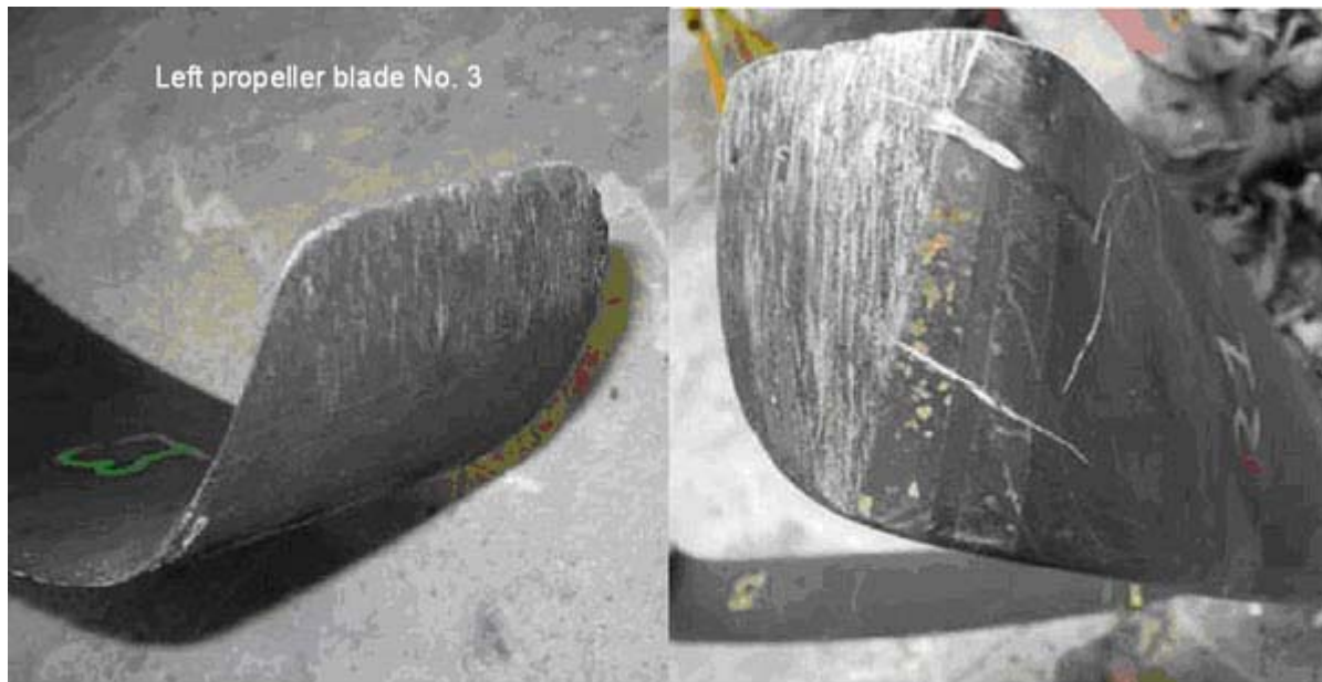
Figure 3 - Spanwise scratches propeller blade (left) versus chordwise scratches (right)
