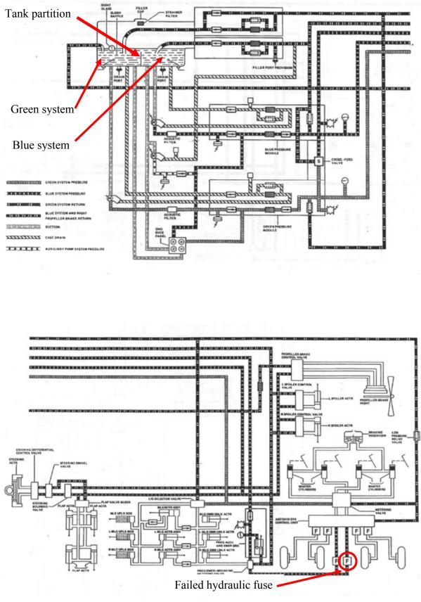
Figure 1 Hydraulic system schematic diagram
