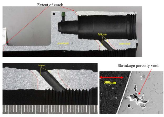
**Figure 3** View of sectioned fuse body showing extent of the crack
