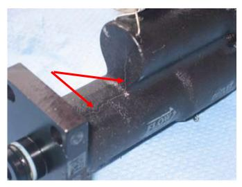
Figure 2 Visible crack on surface of valve body
