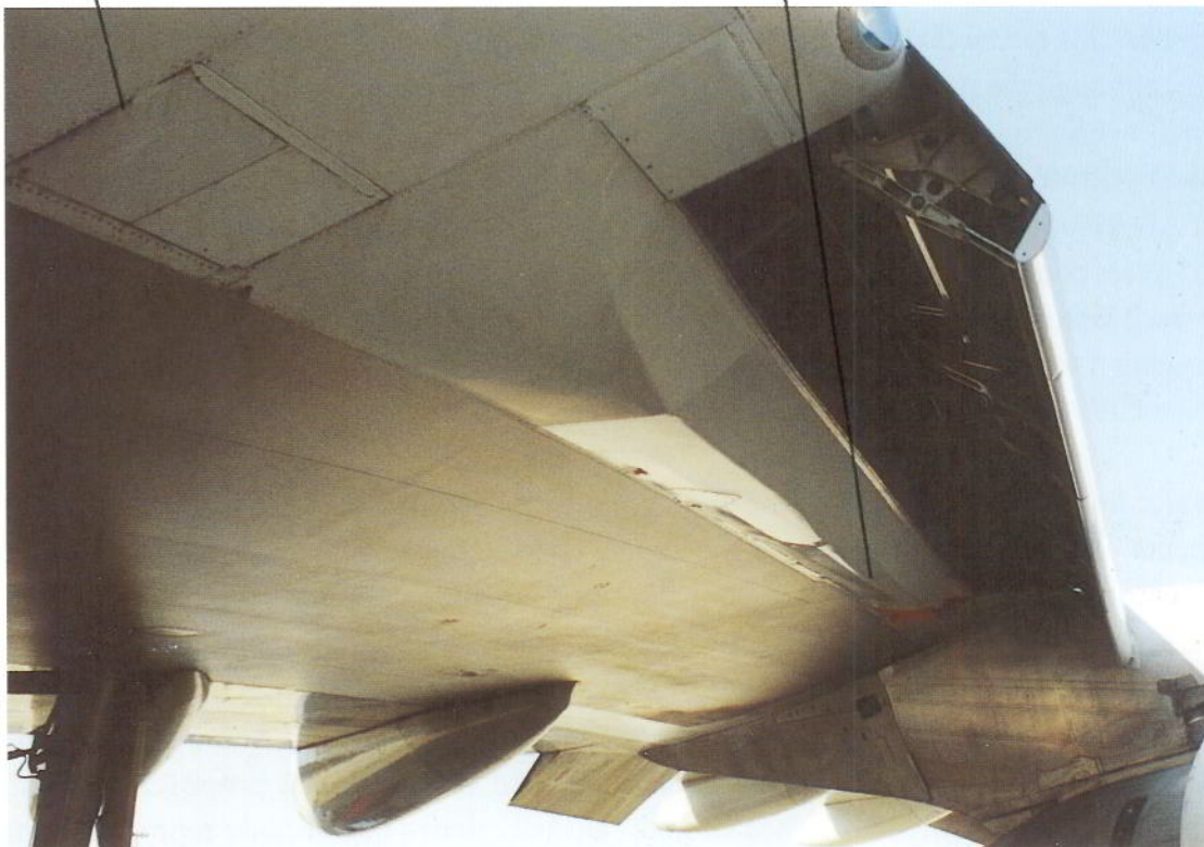
VIEW ON INBOARD LEADING EDGE SHOWING COLLAPSE OF COMPOSITE PANEL AFT OF KRUGER FLAP
