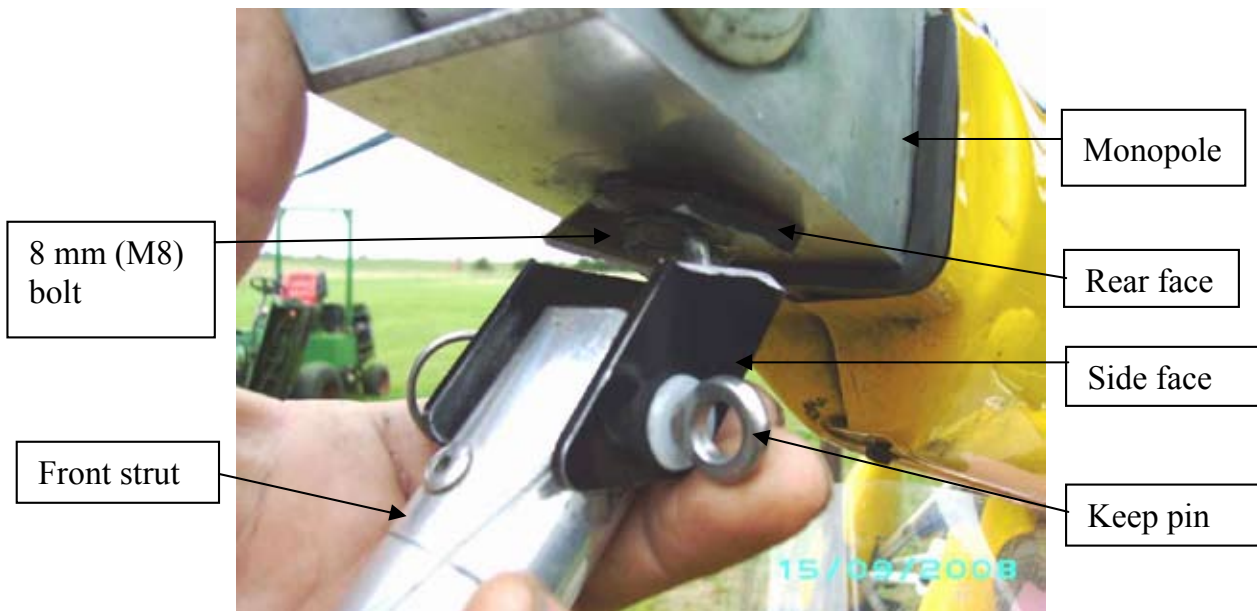
Figure 1 Failed front strut bracket on G-BZMI
