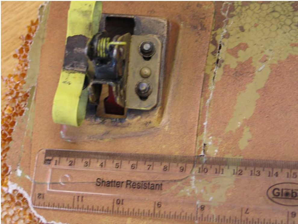
Figure 2 - Engine cowling - Aft latch (inside) and 'anti-chatter' device
