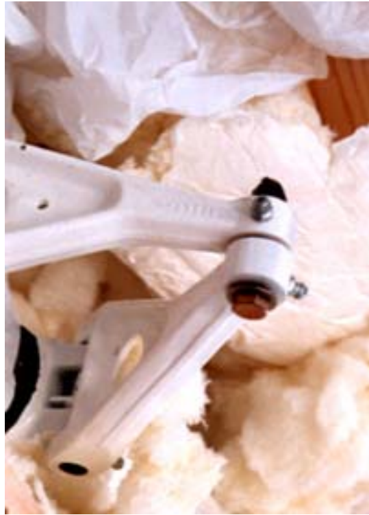
Figure 2: Correct P/N 5045018-1 0.75" washer
