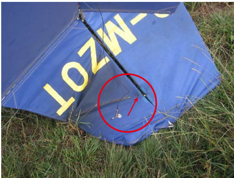
As-found tailplane bracing wires: arrow indicates attachment point on fin
