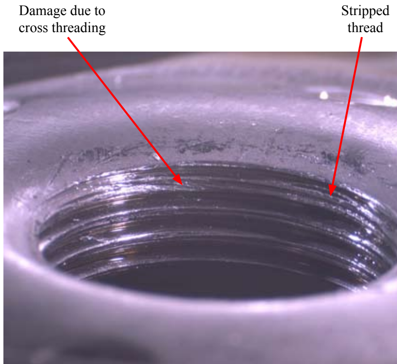
Figure 2 Oil filter thread damage
