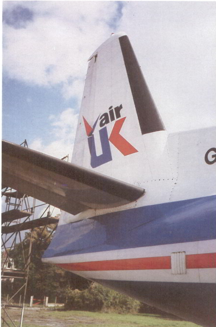
(i) Overall view of vertical tail surfaces with damaged rudder and trim tab
