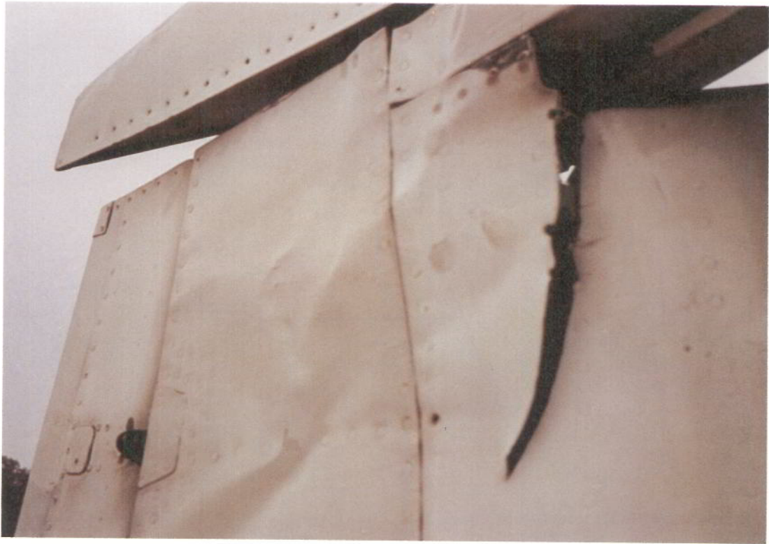
(iv) Damage to rudder structure at top hinge
