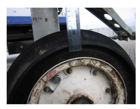
**Figure 9 (left)** Tyre chine, left nosewheel
