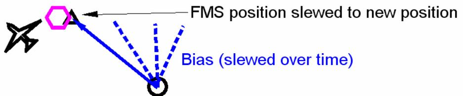
The time taken to slew to the new position is dependant on the flight environment. In this case 2 minutes is typical.
