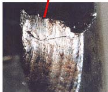
Figure 1. Details of G-TEST oleo strut failure
