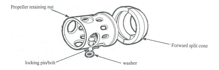
G-BEDA: Diagram showing method of locking Hoffmann propeller nut
