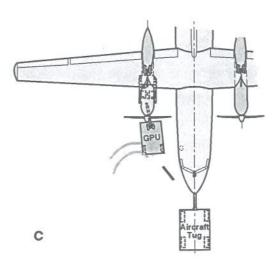
A number of propeller blade strikes on the tractor were evident; the spacing indicated a tractor speed in the order of 6 to 7 mph when it passed through the
