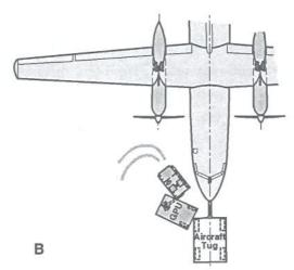
The final orientation of the vehicles and the characteristics of the propeller markings were consistent with the tractor having then travelled forwards, causing the rig to straighten out, before heading nearly parallel with the fuselage axis and passing almost centrally through the lower part of the propeller disc. The rig came to a halt when the front of the damaged tractor collided with the right landing gear drag strut (C).
