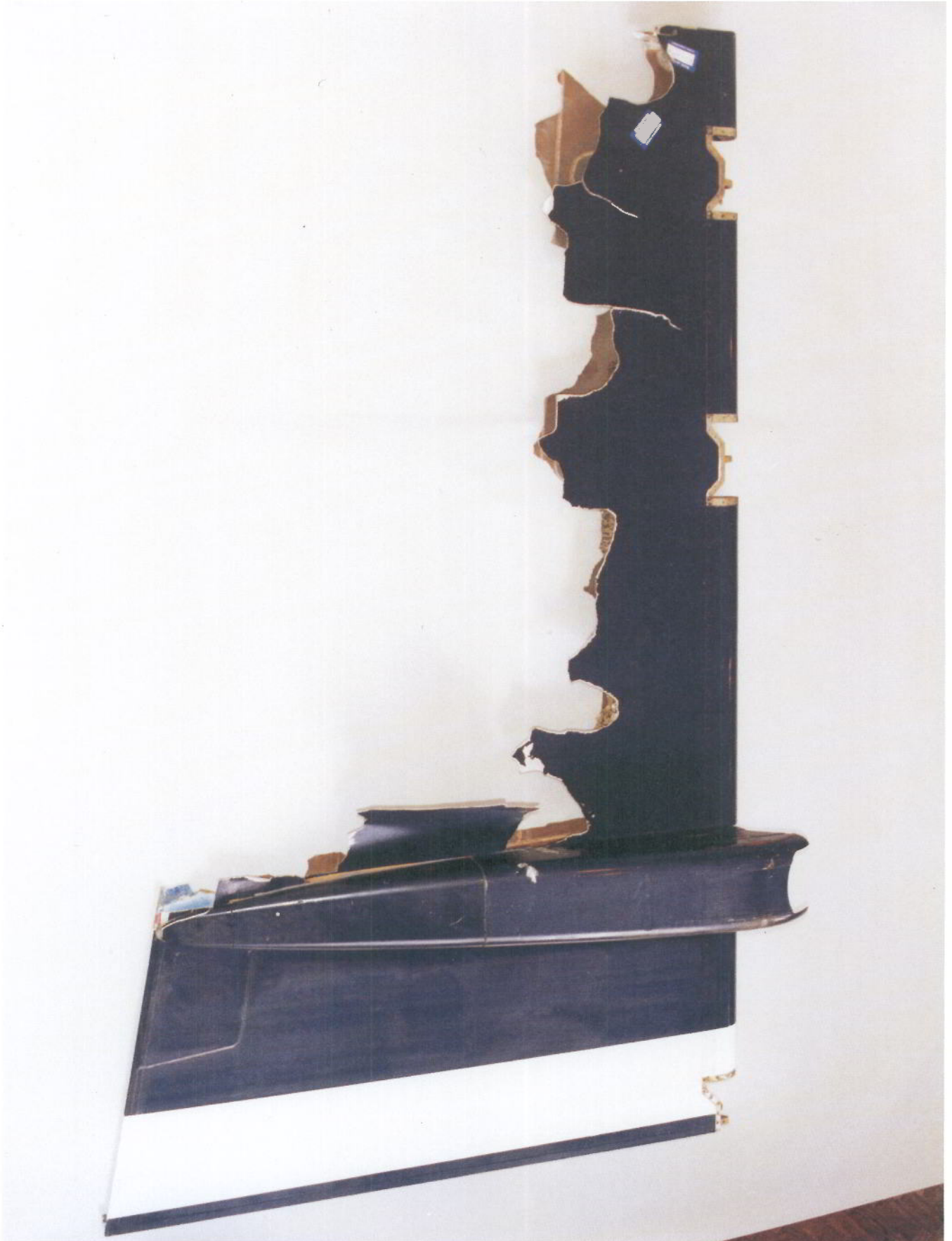
Right Hand Side of Failed Rudder
