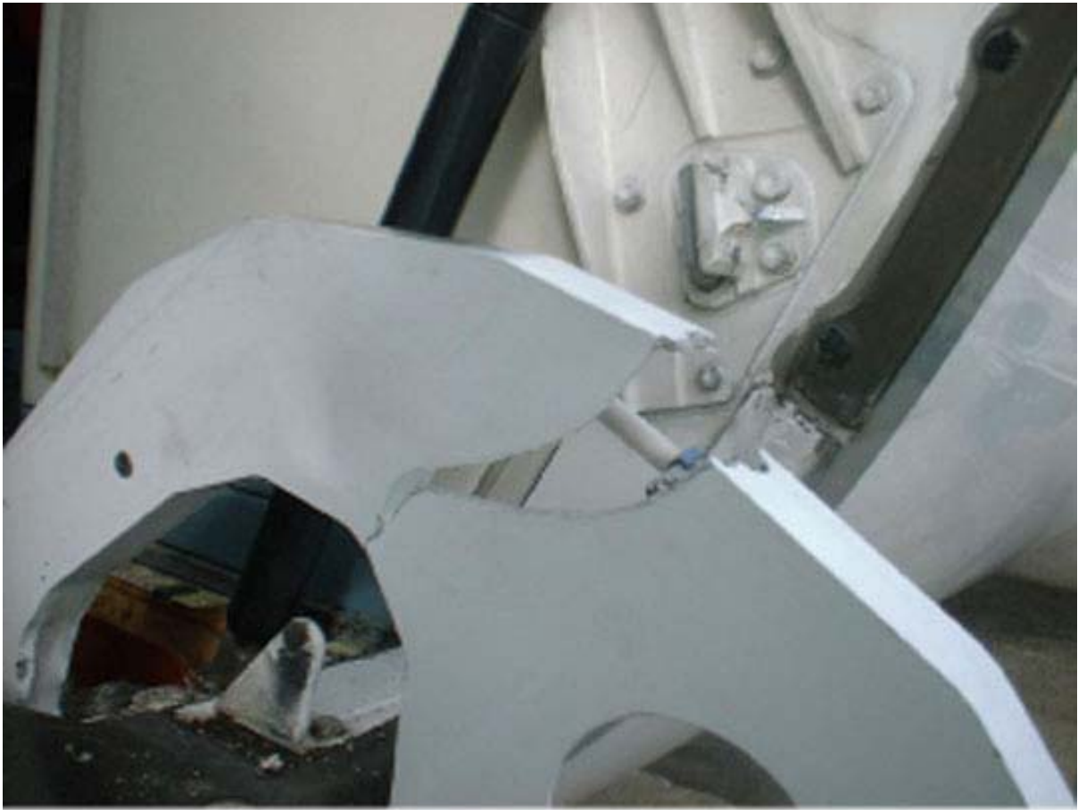
Figure 2 Damaged aft hinge arm
