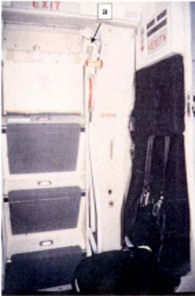
Figure 5 Vestibule with door closed and locked. Note aft facing cabin crew seat, retracted air-stairs and inner door handle (a)
