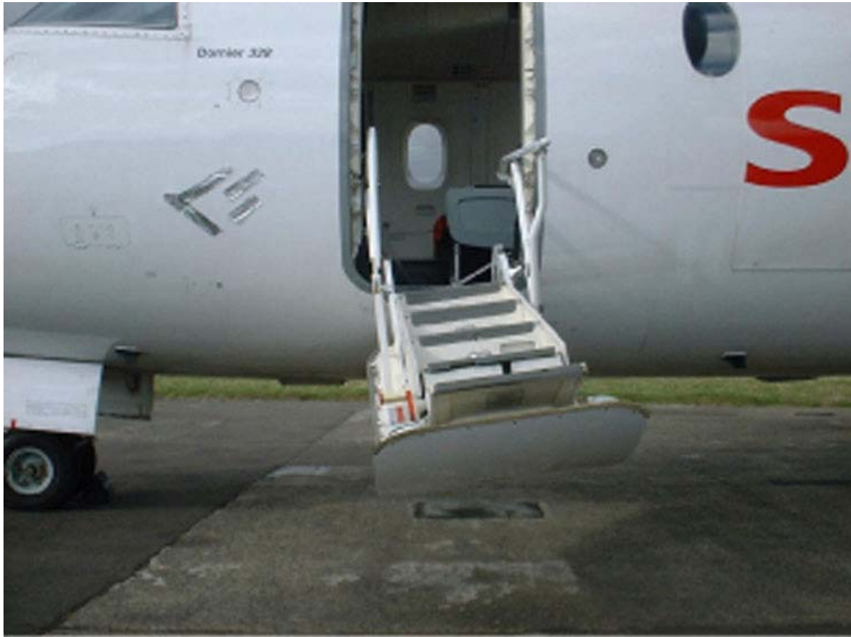
Figure 1 Damaged door on G-BWIR after accident
