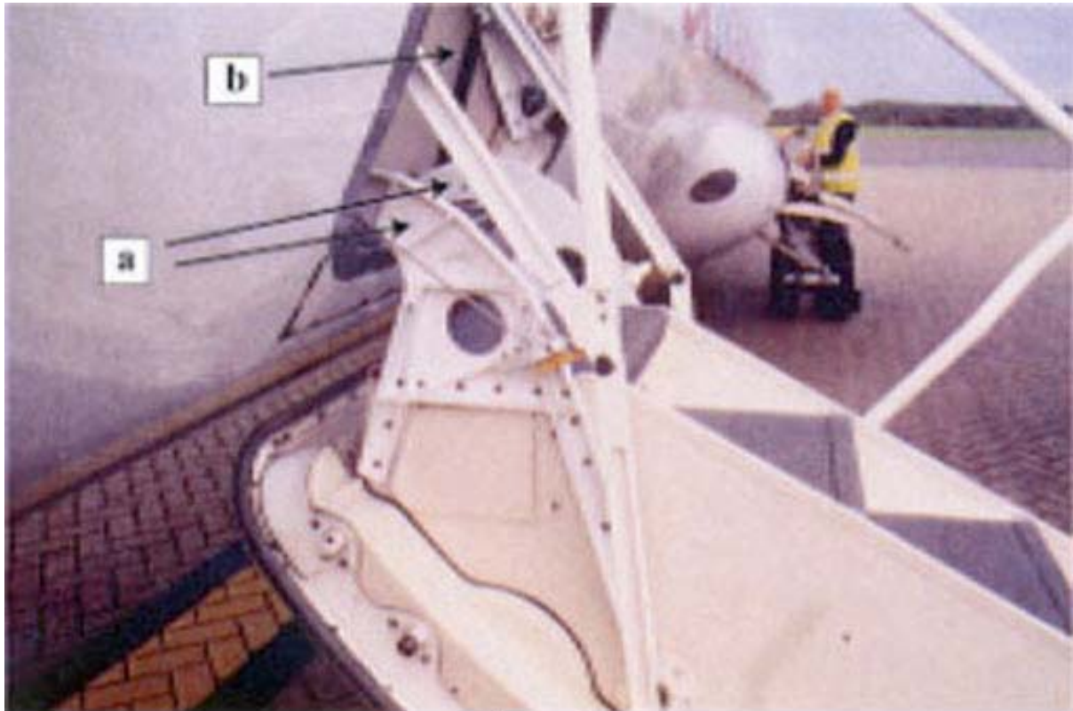
Figure 4 Undamaged example of door fully open, showing hinge arms (a) attaching air-stairs to cabin floor. Damper strut (b) visible within vestibule.
