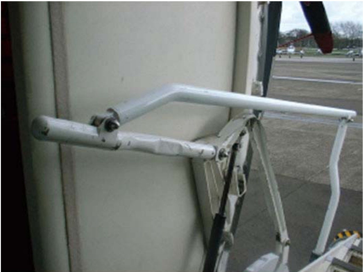
Figure 3 Damaged aft banister restraint system
