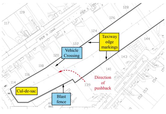
Figure 1 Plan of cul-de-sac, showing pushback details
