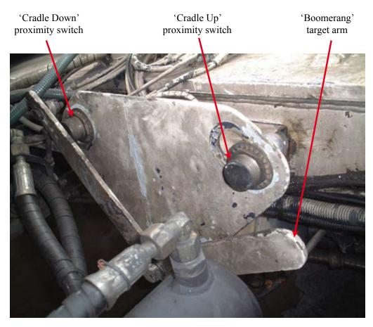
**Figure 5** Cradle position sensor location showing 'boomerang' overtravel
