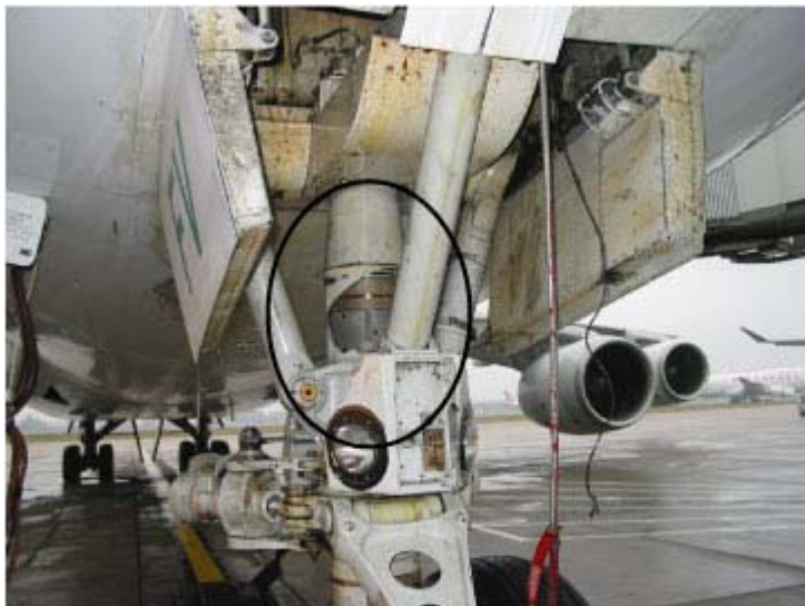
Nose landing gear showing the area of failure
