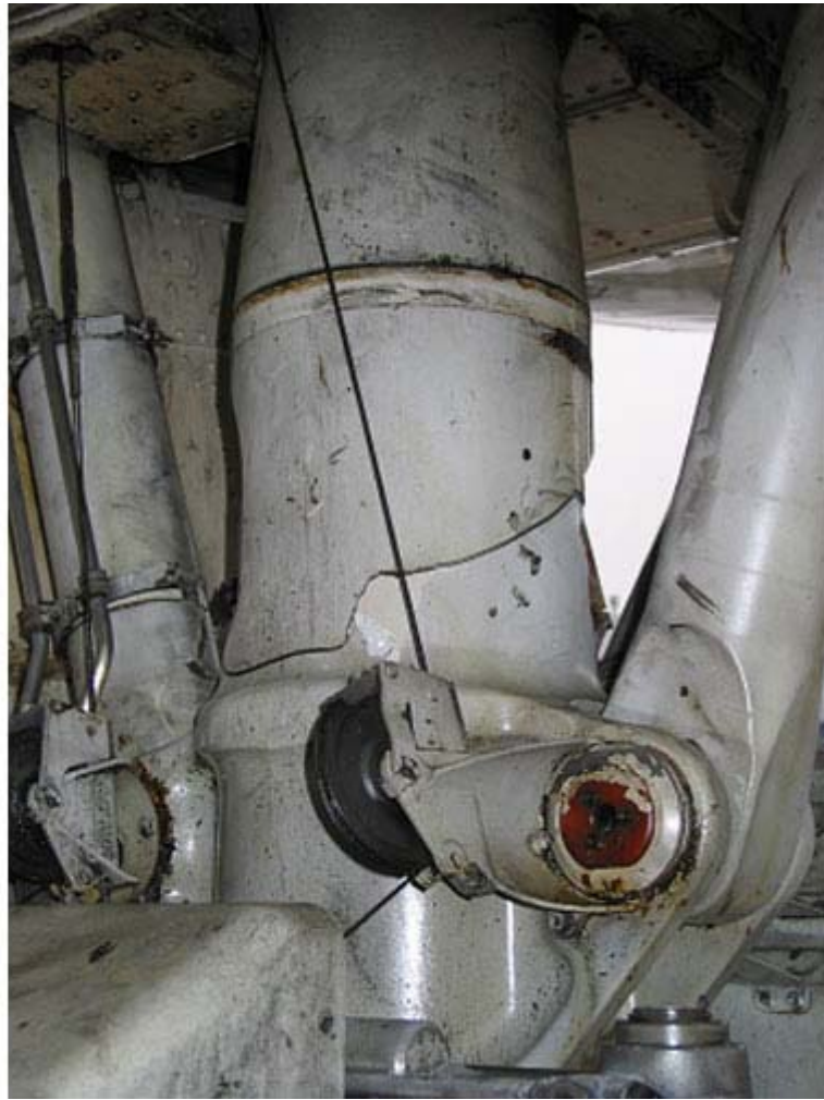
Nose landing gear outer cylinder showing the circumferential failure
