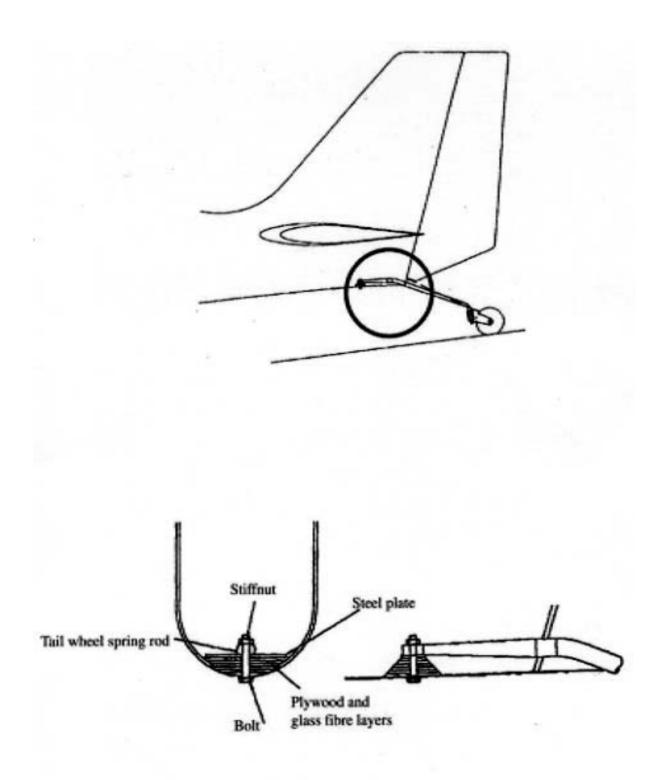
FIGURE 1. Details of Europa G-BWUP tail wheel installation
