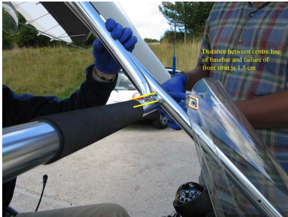
Figure 5 Contact point between basebar and front strut
