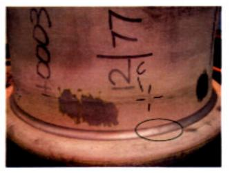
Defects identified in inboard wheel half
