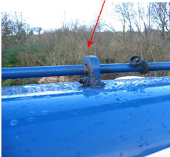
Figure 2 Number 4 bearing and bush as found on G-BYKF with the rubber bush having been released from its location and migrated aft along the exposed tail rotor drive shaft
