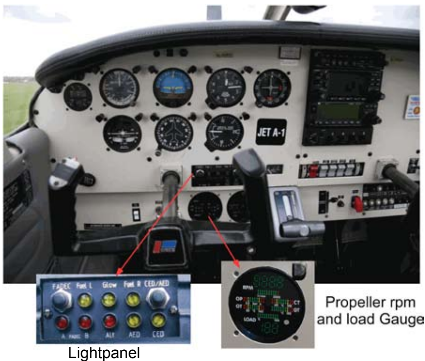
Figure 1 Typical Thielert TAE 125 engine layout instrumentation
