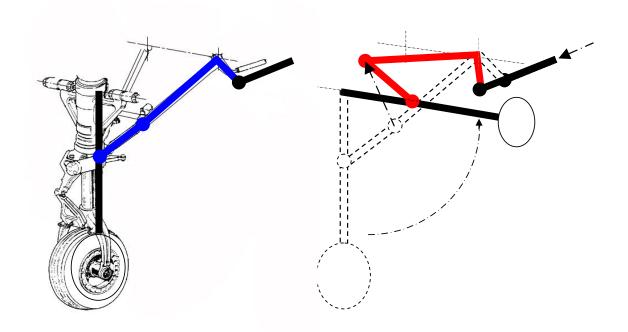
If all of the limit switches close before all of the gear legs are fully down and locked, the motor will stop prematurely, even though the green "down locked" light is illuminated. Dirt collects readily on the nose gear drag link, and rigging tolerances are such that a small accumulation is sufficient to cause the nose gear limit switch to close before the nose gear drag link has locked over centre.
