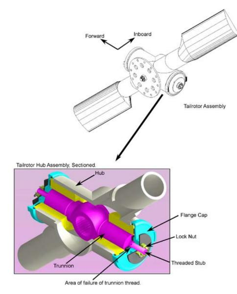
Figure 1 Trunnion assembly and drive
