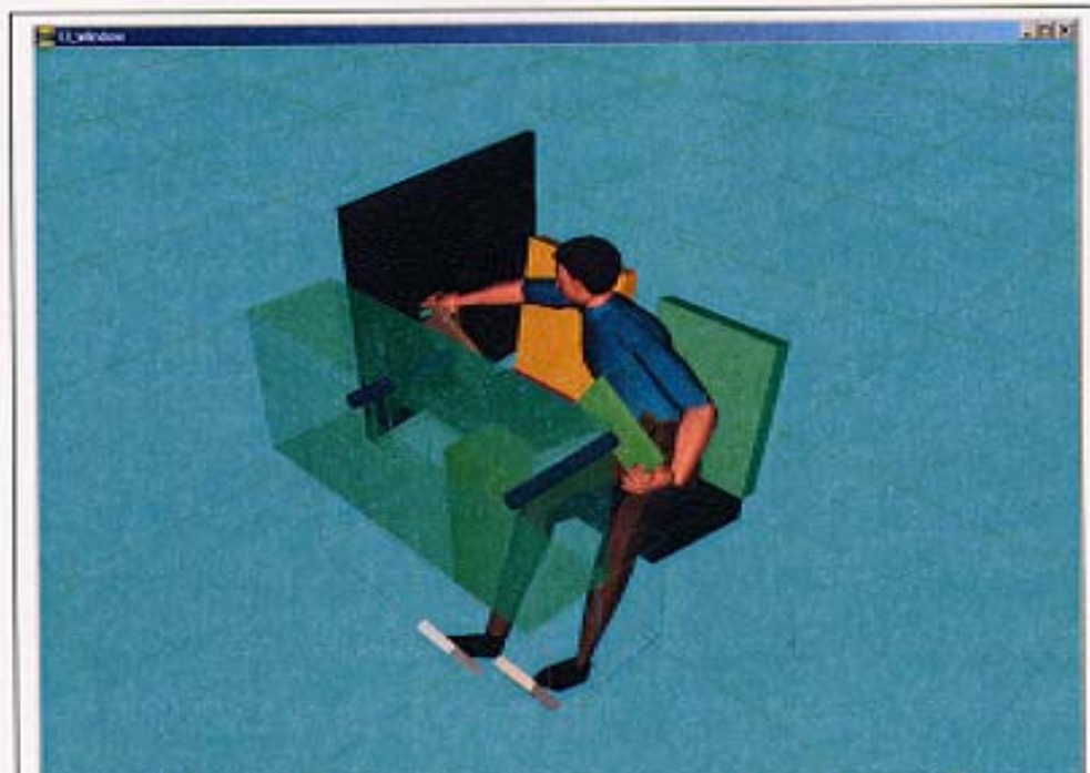
Figure 4: The pilot when pulling the door closed transfers his weight to the right foot, which causes the right rudder pedal to move forward.
