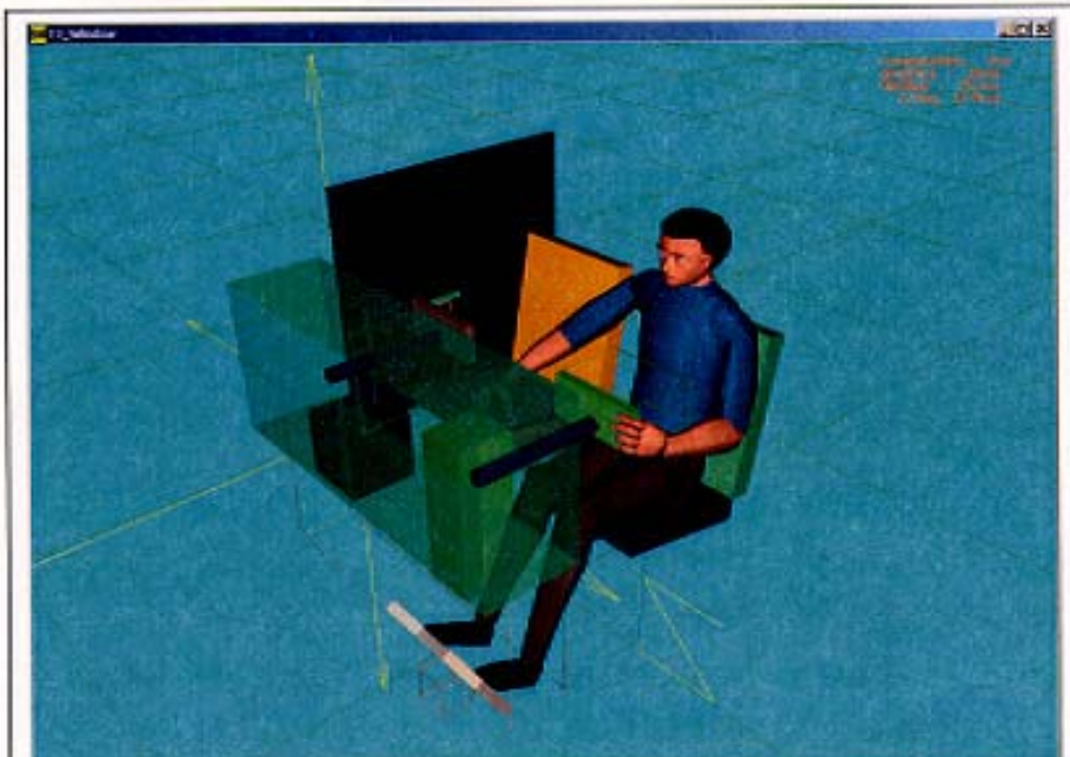
Figure 2: The pilot in the normal seating position left hand on the control yoke, right hand on the throttles and both feet on the rudder pedals.
