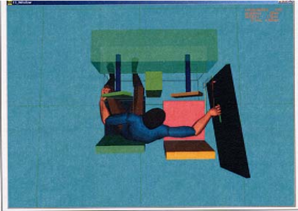
Figure 4: The pilot when pulling the door closed transfers his weight to the right foot, which causes the right rudder pedal to move forward.
