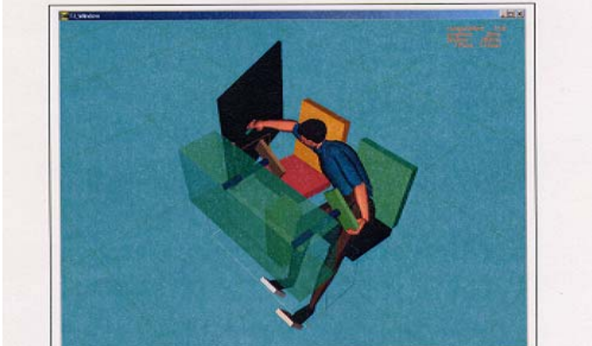
Figure 3: When the pilot reaches across the cockpit and pushes the door into the airflow, his left leg moves to the left with the result the left pedal goes forward. The left hand moves the control yoke down on the left side. This combination of control inputs probably caused the rapid roll to the left.
