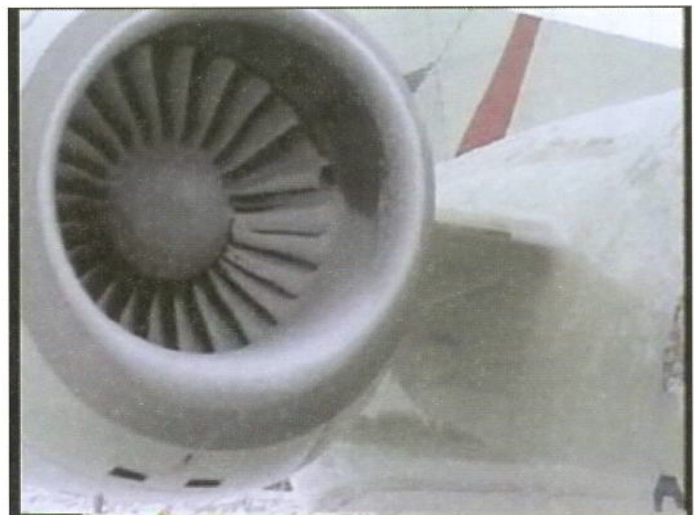
Figure 3 Snow Deposits in Engine Intakes of other Aircraft at Edinburgh during the morning of 27 February 2001
