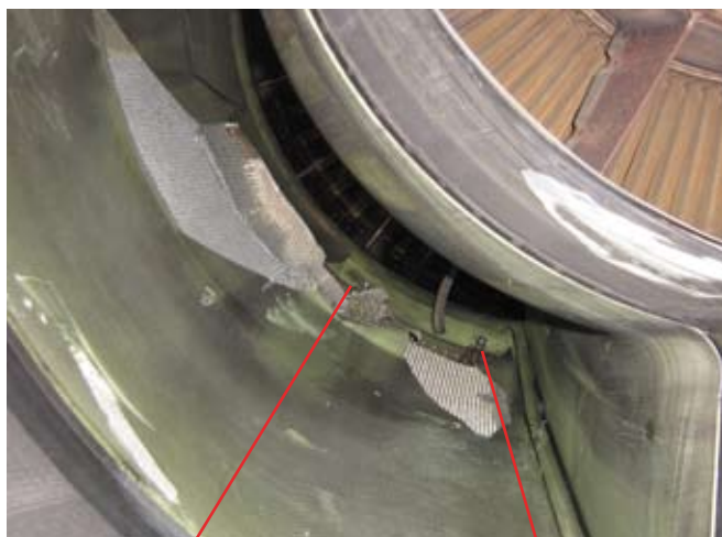
Upper hinge point Lower hinge point
