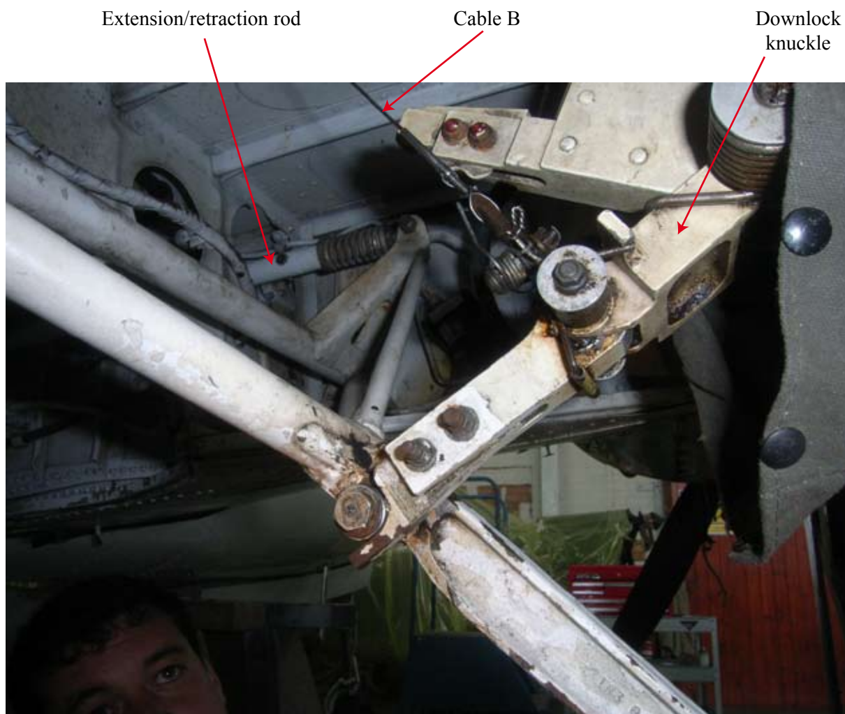
Figure 1 Gear down and locked
