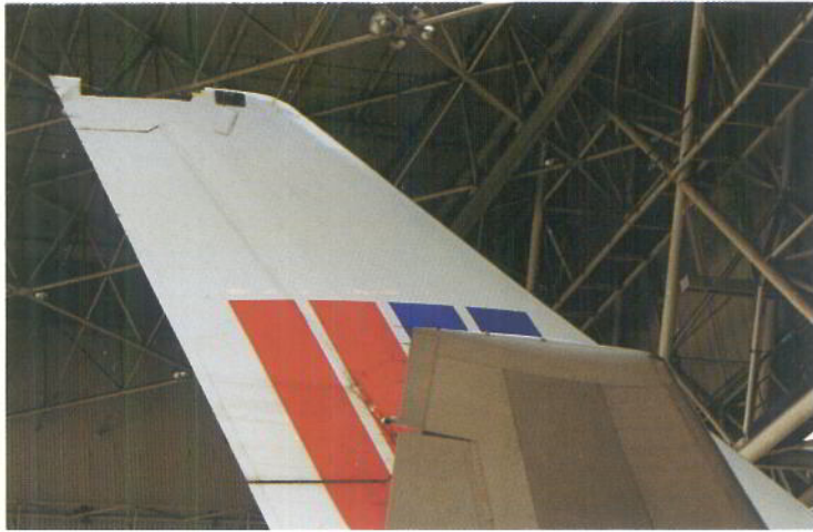
Photo 1 Damage to top of fin as seen from the ground
