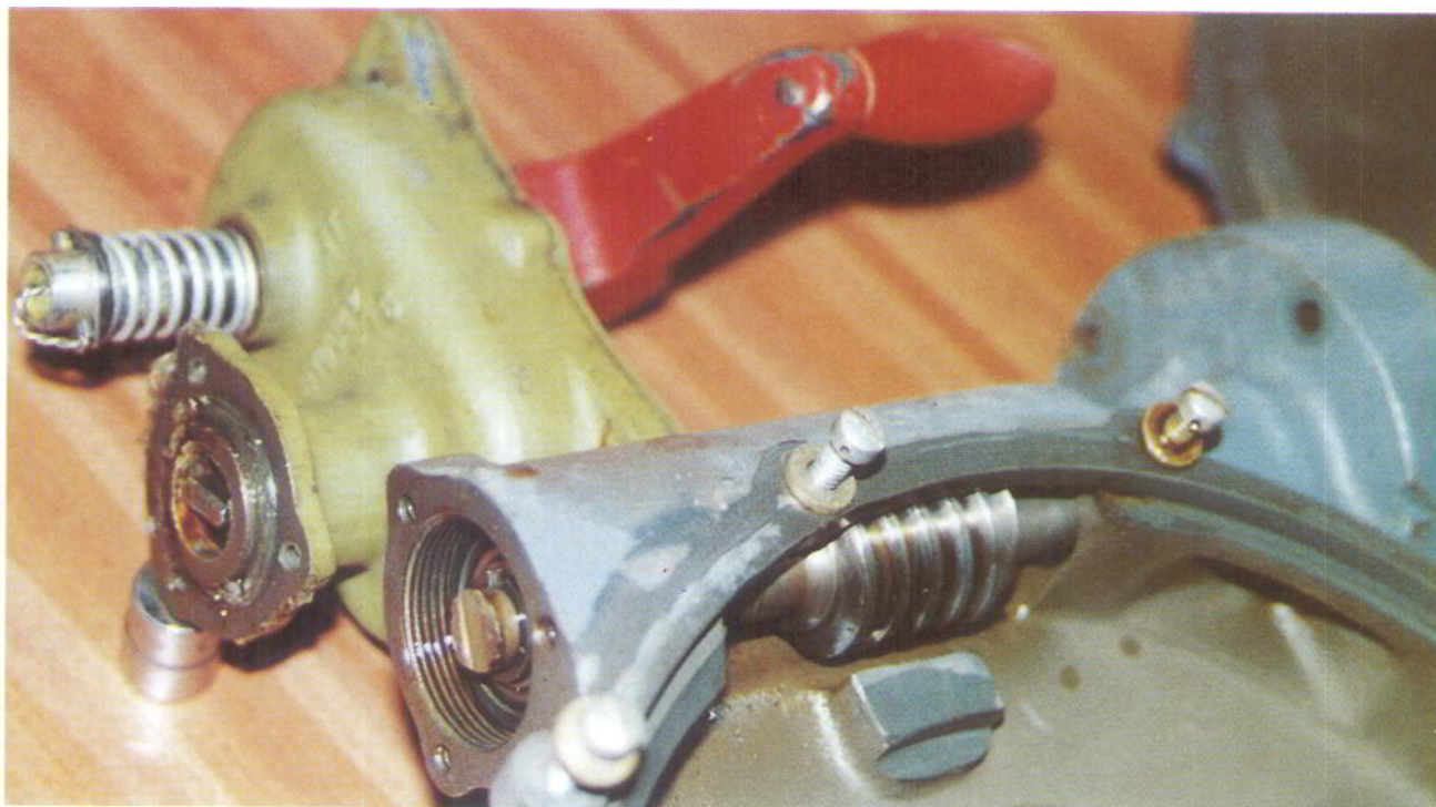
N1024L - Landing gear actuator worm gear shaft and manual drive gearbox (Showing eroded end of worm gear shaft)
