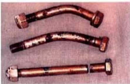
(Photo: H T Consultants) FIGURE 1a. Bolts as received
