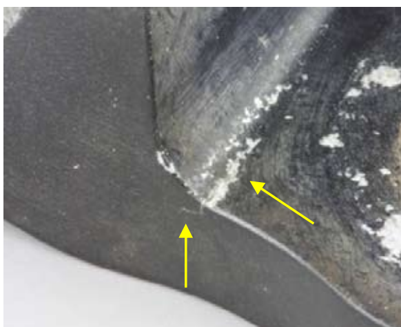
Figure 4 Cracking at base of lugs
