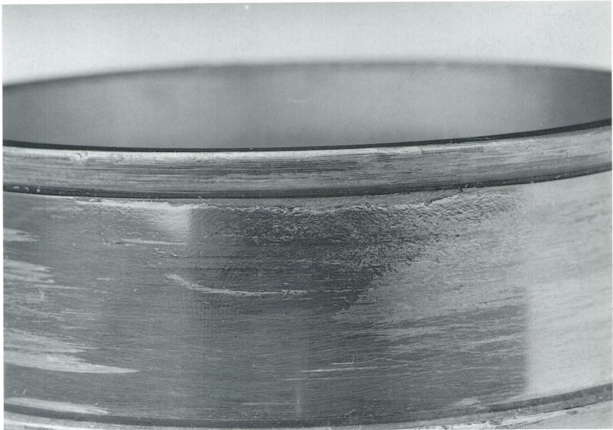
Photograph No.1 Geometric stress concentrations (GSC), a form of fatigue, over 20 degrees of the inner bearing cone, caused by heavy contact with the rollers.
