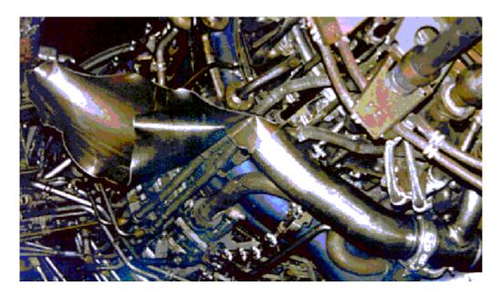
The 14th stage HP air duct on the No 4 engine, part number 9068M-40-G01,had failed causing two blow-out panels to operate, and damageto one half of the reverser shroud. The No 4 reverser deployed,but would not stow. Braking, followed by the aircraft being heldstationary had caused brake overheating which led to tyre failures and brake seizure on the right main gear, and, in order to movethe aircraft, wheels and brake packs had to be changed.
