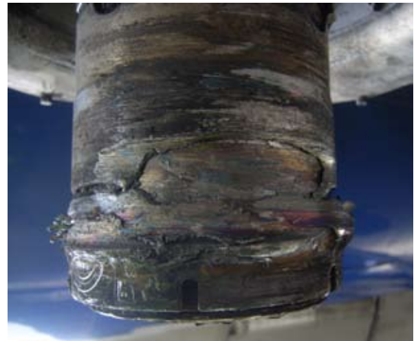
Figure 4 Damage to wheel axle underside (6 o'clock position)
