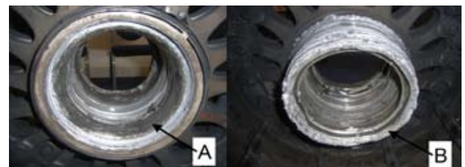
Figure 5 Left: Outer wheel hub showing remains of outer bearing cup (A). Right: Inner wheel hub showing that at (B) the inner bearing hub support and inner bearing cup are missing.
