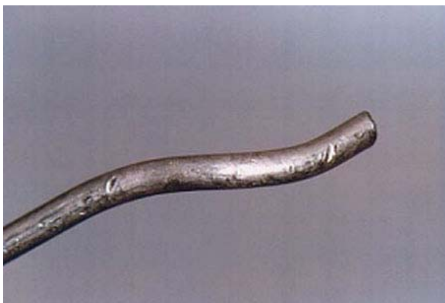
Figure 5. "Joggle" area of mixture cable, showing indentations from cup rim
