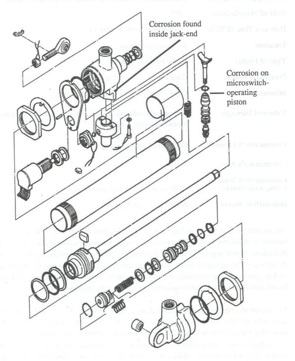
The nose gear was fitted with a Teijin Seiki jack assembly containing a downlock microswitch actuated by a mechanism driven by internal locking keys when the jack was fully extended. On retraction a spring was designed to move the mechanism away from the down position and allow the microswitch contacts to open.
