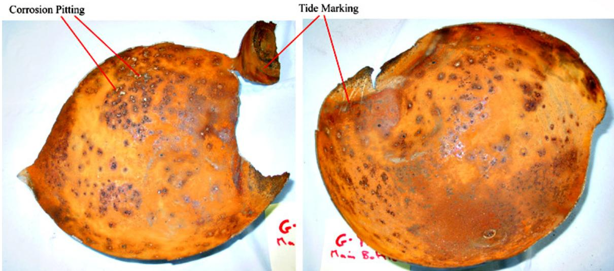
A number of corrosion pits had extended almost to the exterior surface; this was clearly evident in the case of a number of pits that had been bisected by the fracture (Figure 9).
