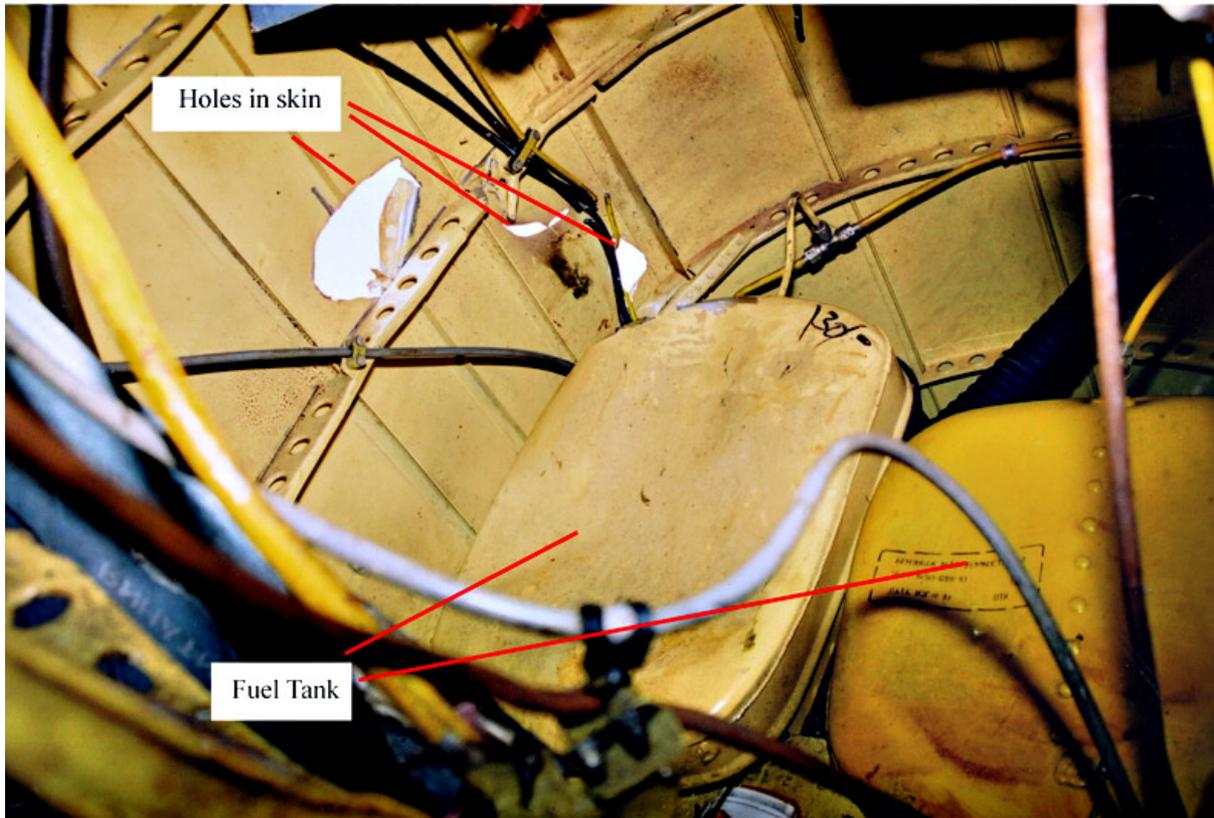
The bottle portion came to rest jammed between the top of the fuel tank and the fuselage structure. A second part, comprising approximately one third of the bottle and including the drain port, had been propelled to the left and had torn an approximately 2 foot diameter hole in the lower left part of the fuselage just aft of the firewall (Figure 3).
