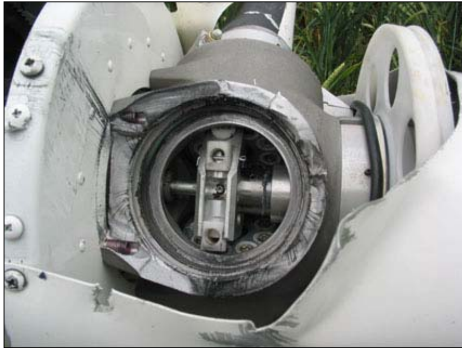
Propeller hub showing fractured No 1 blade socket
