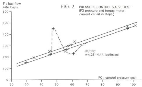
Both points occurred together (*ie* adjacent in the test sequence) at max P3 pressure and max power lever position, but with only moderate fuel demand from the computer - conditions which might be expected to occur in the case of a torque or temperature limited climb. However, it was not possible to determine retrospectively whether these points represented actual deviations from the linear response characteristic or were the result of test instrumentation error.
