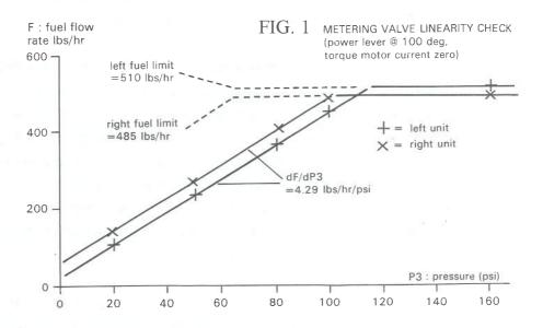
Both units displayed similar response patterns with good linearity (fig.1). There was a rich shift evident in the output of the right unit relative to the left equivalent to approximately 35 lb/hr., but the right unit topped out at a max fuel flow of 485 lb/hr compared with 510 lb/hr for the left unit.
