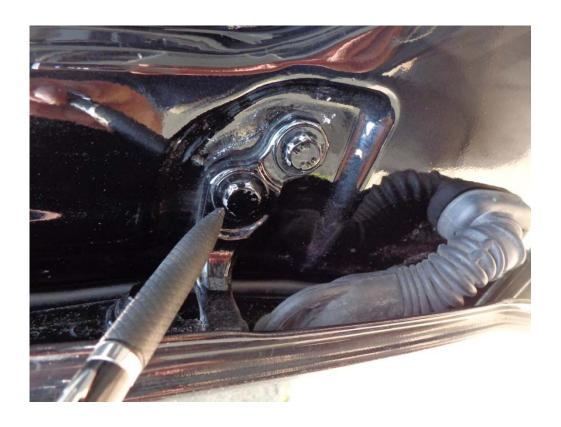
Rounded bolt – Suggesting wrong tool was used in the repair process
