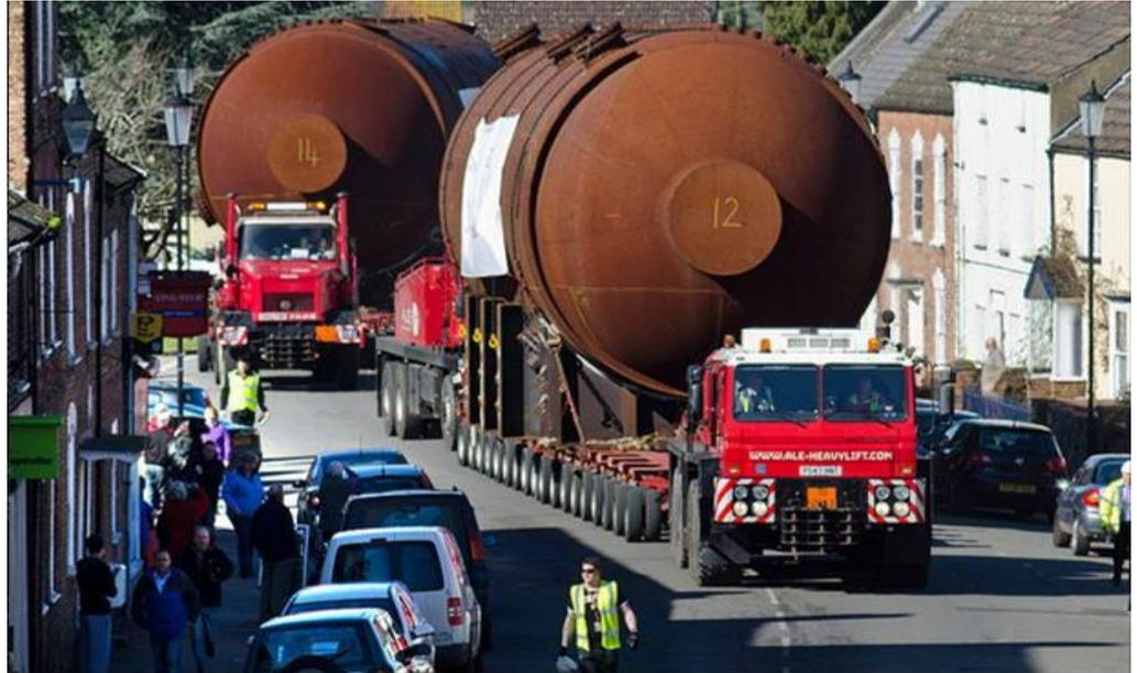
*Under LLWR's landmark Berkeley Boilers project, 2012/13, 15 redundant 300 tonne steel boilers, each 22m long, were transported four miles through Berkeley town centre and on to the coast for shipping to Sweden. Around 95% of the steel was recycled for reuse.*
