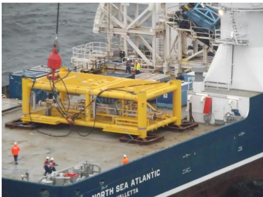
**Figure 3.7: Example of a Typical Manifold on the Back of an Installation Vessel**
