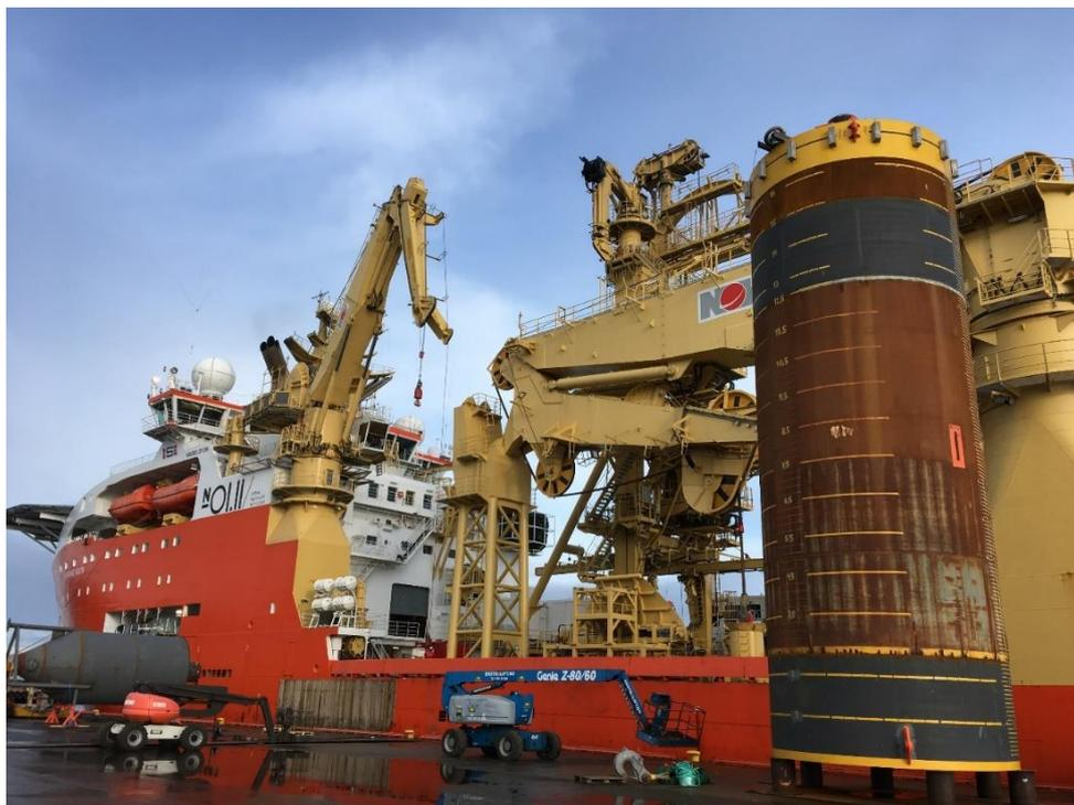
**Figure 3.4: CAN-ductor for the Previously Drilled Cambo 5Y Well on the Quayside, Awaiting Deployment**
